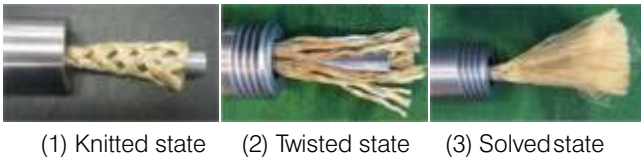
Fig. 6: Various disengagement states of fiber rope end
