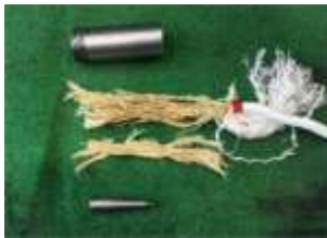
Fig. 4: Breaking state of fiber rope
