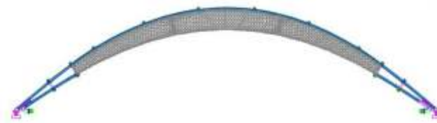
Figure 3: Hybrid system ready to attach membrane (erection process)
