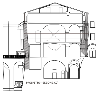
Figure 5: Provisional interventions carried out on SE and SW wings: connection of the internal and external façades by means of steel cables and steel frames against the façades.
