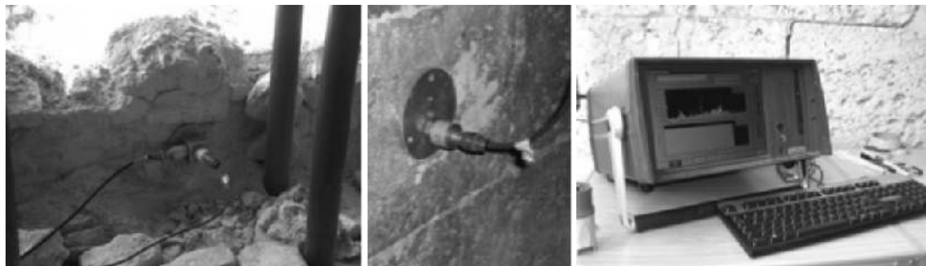
Figure 13: Accelerometers on walls and the acquisition system
