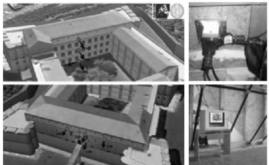
Figure 15: The Spanish fortress: left - localization of the acceleration transducers; right – base acceleration transducers (CH1, 2) and acquisition unit.
