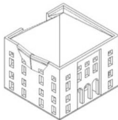
Figure 3: Out-of-plane overturning of the upper part of the main façade (South-East side)
