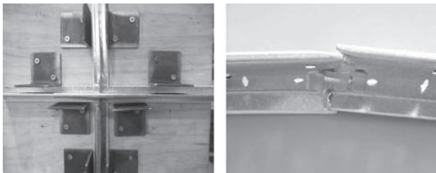
Figure 6. Failure mode in a compression test specimen
